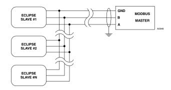
Individual Eclipse units are wired as shown below. Note the inclusion of the end-of-line termination resistor.
