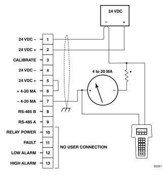
\*TOTAL LOOP RESISTANCE = 250 OHMS MINIMUM, 600 OHMS MAXIMUM. DO NOT INSTALL RESISTOR WITHIN PIRECL ENCLOSURE IN EEX @ APPLICATIONS.
