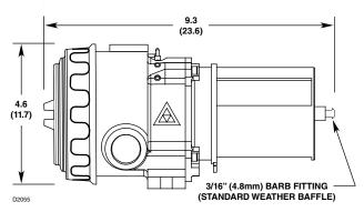
Figure 2—Dimensions of Eclipse Detector in Inches (Centimeters)
