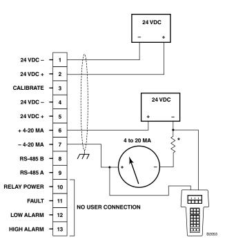
\*TOTAL LOOP RESISTANCE = 250 OHMS MINIMUM, 600 OHMS MAXIMUM. DO NOT INSTALL RESISTOR WITHIN PIRECL ENCLOSURE IN EEX e APPLICATIONS.
