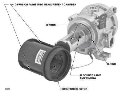
Figure 17—PointWatch Eclipse with Baffle Removed
