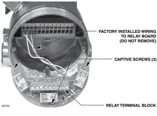
Figure 3—Eclipse Wiring Termination Compartment with Optional Relay Board Removed
