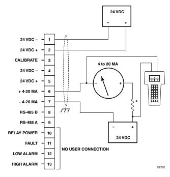
\*TOTAL LOOP RESISTANCE = 250 OHMS MINIMUM, 600 OHMS MAXIMUM. DO NOT INSTALL RESISTOR WITHIN PIRECL ENCLOSURE IN EEX e APPLICATIONS.
