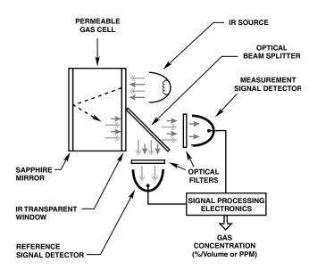
Figure 1—Measurement Scheme for Infrared Gas Detector
