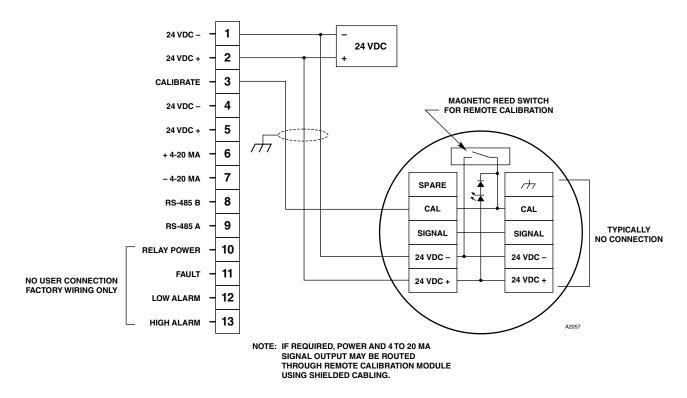
Figure 13—PIRTB Wired to PointWatch Eclipse
